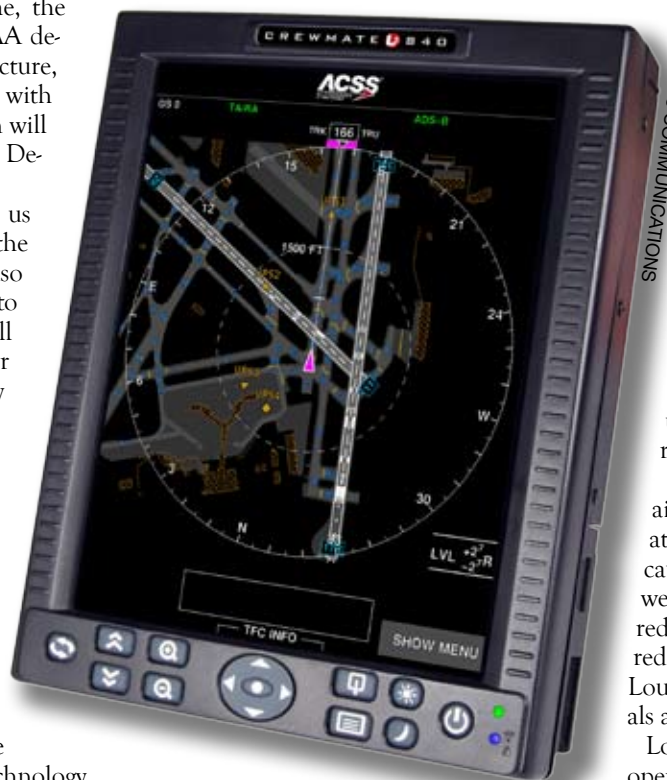
ACSS's SafeRoute suite of ADS-B In software applications includes an airport moving map showing airborne and ground traffic, as here on an electronic flight bag.
