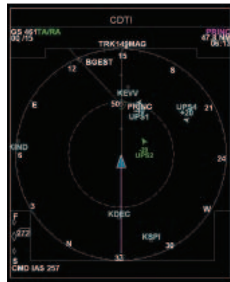
ACSS merging and spacing software commands the pilot (see "own-ship" position at blue triangle) to merge behind UPS 2 at PRINC waypoint (indicated by outline around UPS 2's green icon). However, the aircraft is flying at 272 kt., faster than the 257 kt. commanded by software (note fast-slow indicator lower left).
