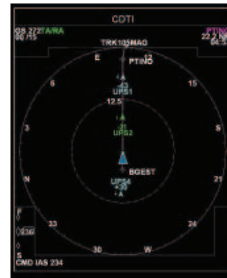
This scenario shows proper in-trail spacing with "own-ship" aircraft (blue triangle) flying behind UPS 2 at 236 kt. compared with commanded IAS of 234 kt. on fast-slow indicator (lower left).
